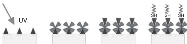
Figure 16 Schematic illustrating the chemistry used to specifically immobilize peptides to lithographic features. Photobiotin (triangles) was activated with UV light to initiate binding. Biotin was next coupled to the surface (crosses), followed by the idoacetamide-functionalized biotin (triangles) and the final cysteine containing peptides. Reprinted with permission from Dinca et al. (2008) (copyright 2008 American Chemical Society).
